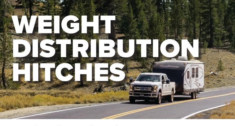
A WEIGHT DISTRIBUTION HITCH provides safe and level towing. It allows the trailer weight to be evenly distributed across the axles of your tow vehicle. Without a WDH, extra weight is put on your tow vehicle's rear axle. Limited weight on your front axle creates light steering and potentially dangerous driving conditions.
